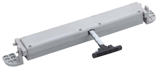
SUPERNOVA chain actuator Force 300N - stroke 400mm or selectable stroke (0-300 mm)
